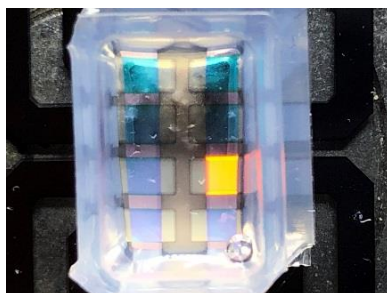
Supplementary Figure 10. Stability test under exposure to cell culture medium. Photograph of an OLED with TFE barrier and a silicone chamber (ibidi) attached that confines culture medium to OLED pixel area and avoids interference of the liquid with the electrical contacts.
