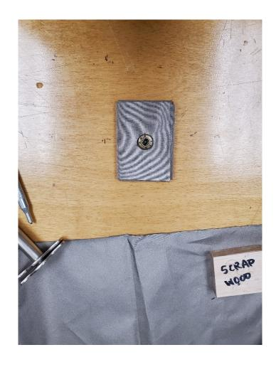
Cut thin strips of low profile Velcro (hook end) and use fabric glue to glue them to the electrode as shown in the picture. You are finished with making the electrodes.
