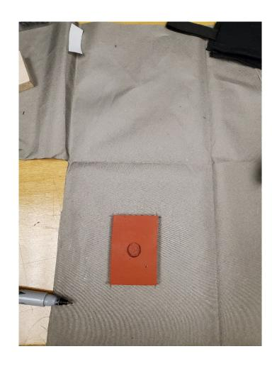
Connect the lines you made in the corners of the silicone rubber and draw lines extending out towards the edge of the fabric as shown in the picture.
