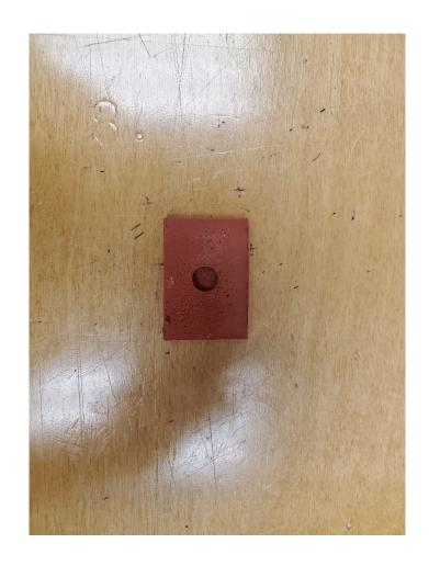
Locate the ferrous fabric and place the silicone rectangle on top of the fabric. The fabric piece should be approximately  $4 \frac{1}{2}$ " x  $6 \frac{3}{4}$ ". Make marks on the corners of the silicone rubber as shown in the picture.
