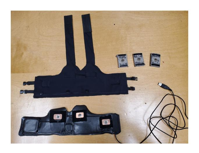
Start by opening the fabric portion of the vest and guiding the USB cable inside the vest to exit out the lower right portion of the vest. Pull the slack out of the cable until most of the cable is through the vest as shown in the pictures.
