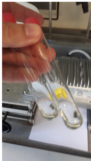
Fig. S167. Homogeneous reaction mixture consisting of monomers alkoxybutenolide B2-5 – di(ethylene glycol) divinyl ether (1:0.5 ratio) and 3 mol% of Omnirad 819 (bis(2,4,6-trimethylbenzoyl)phenylphosphine oxide) before application (left). Resulting alkoxybutenolide coating after UV-curing for 5 min ( \lambda_{\text{irr}} = 395 nm) (right).
