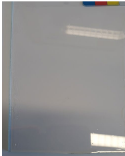
Fig. S167. Homogeneous reaction mixture consisting of monomers alkoxybutenolide B2-5 – di(ethylene glycol) divinyl ether (1:0.5 ratio) and 3 mol% of Omnirad 819 (bis(2,4,6-trimethylbenzoyl)phenylphosphine oxide) before application (left). Resulting alkoxybutenolide coating after UV-curing for 5 min ( \lambda_{\text{irr}} = 395 nm) (right).
