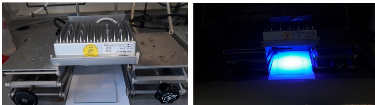
Fig. S166. Irradiation setup, LED Beacon above glass plate with uniform film of reaction mixture (alkoxybutenolide B2–5 – di(ethylene glycol) divinyl ether (1:0.5 ratio) and 3 mol% of Omnirad 819 (bis(2,4,6-trimethylbenzoyl)phenylphosphine oxide (left), irradiation setup in action ( \lambda_{\text{irr}} = 395 \text{ nm} ) (right).
