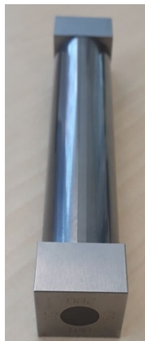
Fig. S165. Byk applicator for film formation.
