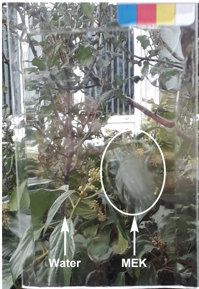
Fig. S173. Methoxybutenolide coating BP4 subjected to standardized spot tests, droplet of water removed after 1 hour, droplet of 2-butanone (MEK) removed after 1 min. Water has no effect on coating resulting in no visible defects. MEK has a minor effect on coating resulting in very slight discoloring. Coating formation conditions: alkoxybutenolide – di(ethylene glycol) divinyl ether (1:0.5 ratio), Omnirad 819 (3 mol%), UV irradiation ( \lambda_{\text{irr}} = 395 \text{ nm} ), 5 min.
