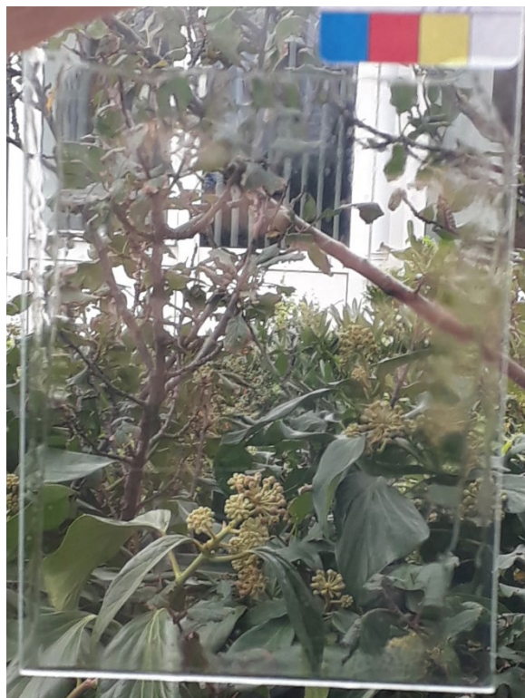
Fig. S172. Uniform transparent alkoxybutenolide coating on glass surface (example: hexyloxybutenolide coating HP4 ). Coating formation conditions: alkoxybutenolide – di(ethylene glycol) divinyl ether (1:0.5 ratio), Omnirad 819 (3 mol%), UV irradiation ( \lambda_{\text{irr}} = 395 \text{ nm} ), 5 min.
