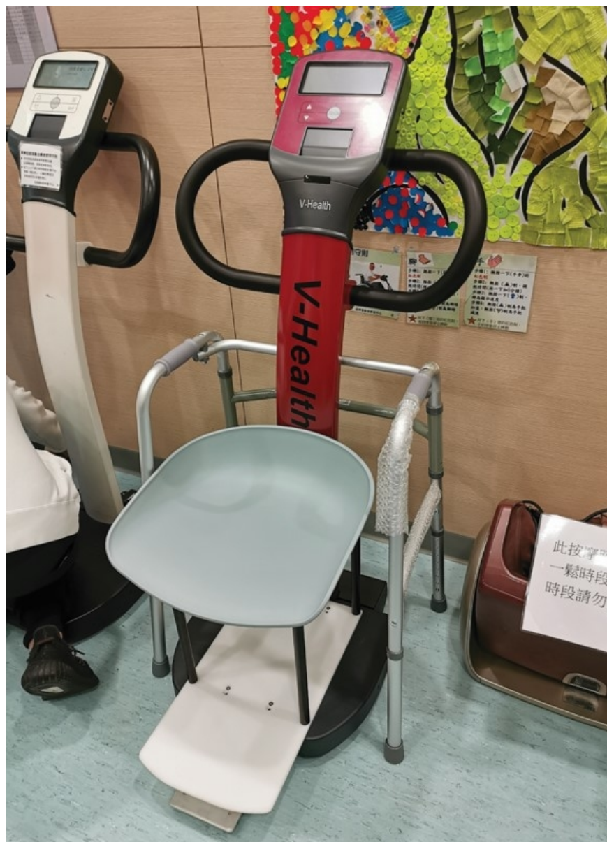
A vertical-oscillating vibration platform modified to provide a seating place for the research subject to receive the 20 min/day treatment. This representative vibration platform is installed in a community centre situated in a public housing estate with 6692 units/families in the Shatin district of Hong Kong.
