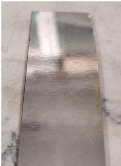
Figure S50. Stainless steel substrate photograph post-peel test show the difference between (A) an adhesive mode of failure with no polymer residue left over and (B) a cohesive mode of failure with visible polymer residue on the substrate.
