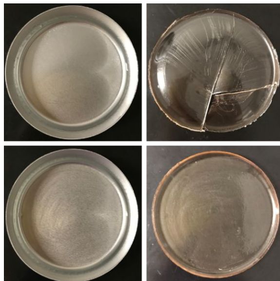
Figure S1. Photos of the HDA monomer with 3 wt% photo initiator (upper left) and its UV cured polymer (upper right), the BPA monomer with 3 wt% photo initiator (lower left) and its UV cured polymer (lower right).
