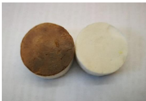
Fig. S11 Photograph of the pure CNF aerogel (left), and CNF@Al-MIL-53 aerogel (right) after the high-temperature thermal insulation test. The surface of the aerogels was put on the heating stage (300 °C) for 100 min
