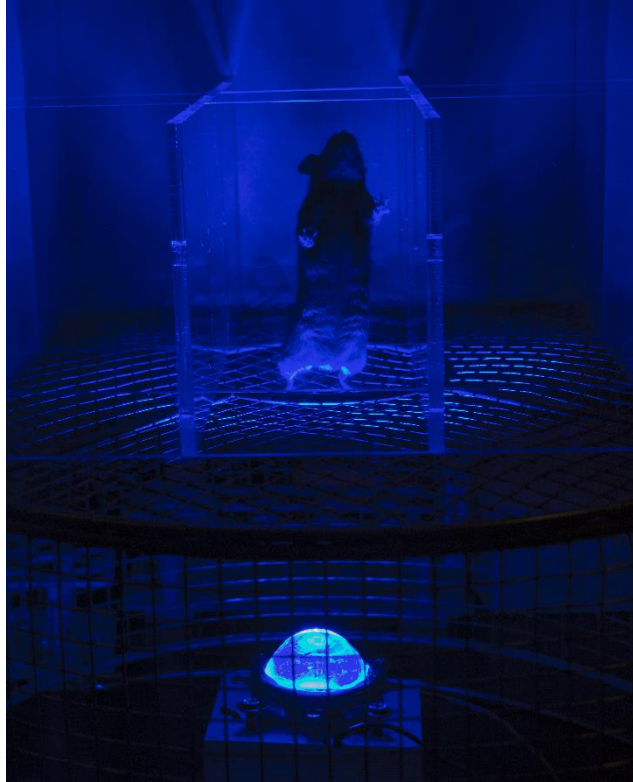
Figure S11. Mouse illumination device. Mice are illuminated with a LED (50 W, 45 m l L, 460-470 nm, with the light angle 60°) which was obtained from Shenzhen Kiwi Lighting Co. Ltd. This integrated LED contains 50 small LED (1W) beads. The light intensity was measured at a wavelength of 465 nm using an optical power meter (Q8230; Advantest) according to the manufacturer's operating specifications. (Photo Credit: Deqiang Kong, East China Normal University)
