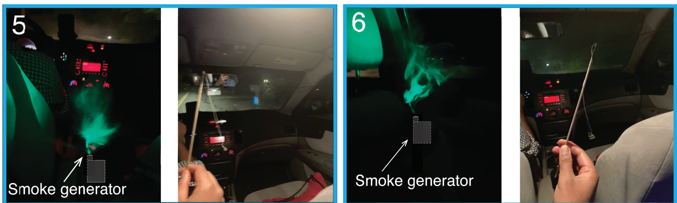
FIG. S-3. Field test images obtained using smoke generator (left sub-figure) and flow wand (right sub-figure). The images in sub-figures (5) and (6) were taken near the circulation zone, given in blue in Fig. S-1. The smoke diffuses very gently in this zone, indicating a low air flow speed. Similarly, the flow wand fails to catch the wind, and stays almost vertical, suggest a stagnant region of air. This field test provides a validation of the results from the steady RANS simulations. [photo credit: Varghese Mathai]
