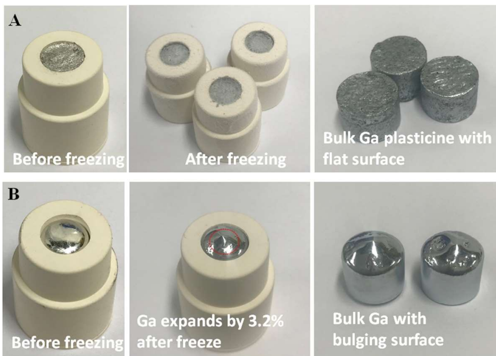
Figure S6. Photographs showing the effect of freezing on both GalP (G-O) and pure Ga. (A) GalP (G-O) does not exhibit any volume change upon freezing and its molded shape is unchanged. (B) In contrast, the pure Ga forms a rounded top due to the high surface tension and expands during freezing, creating the 'spike' visible in the ingot (red circle).
