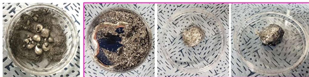
Figure S10. Photos showing how the particle size affects the incorporation. (A) silicon carbide, (B) diamond and (C) graphite into liquid Ga. When the particle size is large, a non-metallic particle is able to mix with Ga to form a putty-like composite.
