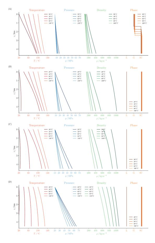
Fig. S1. Wellbore path of CO<sub>2</sub> injection. Profile of temperature, pressure, density and phase of CO<sub>2</sub> during isenthalpic injection for a wellhead pressure of (a) 5 MPa, (b) 7.5 MPa, (c) 10 MPa and (d) 20 MPa. The phase curves appear slightly shifted to improve visibility in case of superposition, with symbols indicating liquid (L), gas (G) and supercritical (SC) phase.
