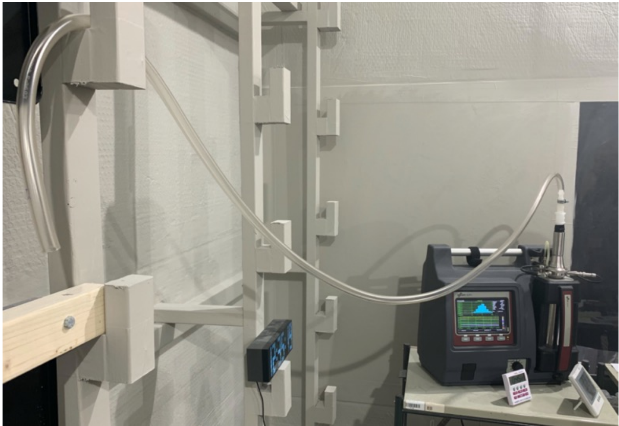
Figure S2: Position of silicone tube relative to the particle sizer.
