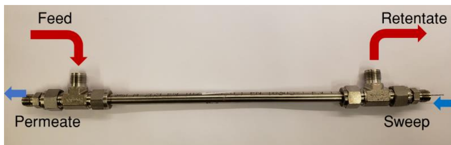
Supplementary Fig. 18. A representative module used for mixed gas permeation measurements operated in a counter-current flow pattern. Gas is fed from the shell side, and the permeate gas comes from the bore side using argon as sweep gas.
