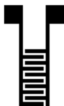
Fig. S10 Layout of an interdigitated Laser-Induced-Graphene electrode on polyimide substrate
