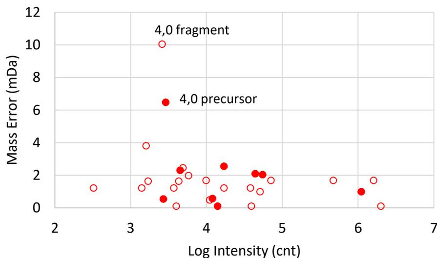
Figure S5: QToF mass error as a function of signal intensity. Filled circles represent precursors, open circles represent fragments. Mass error does not exceed 4 mDa for any data having signal intensity  $\geq 10^4$ .
