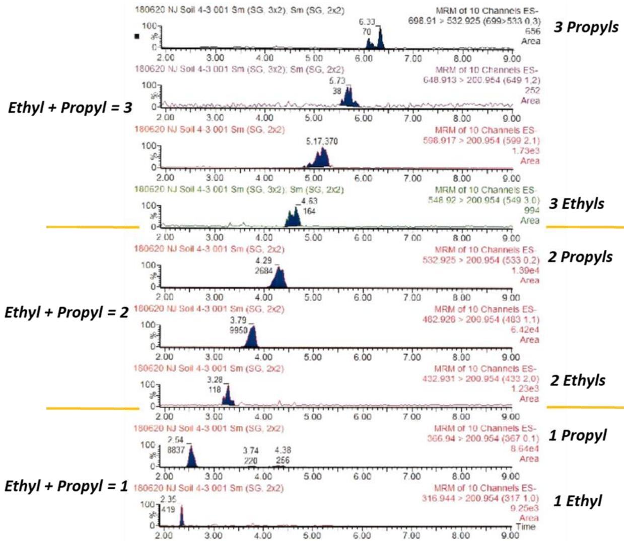
Figure S4: Example tandem mass-spectrometer chromatograms of nine C10 PFAS congeners detected in NJ samples, Soil Sample SS8 shown here. Note congeners elute in order according to molecular mass, small to large.
