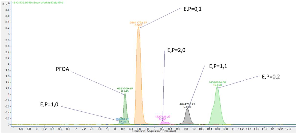
Figure S3: MS<sup>c</sup> mass chromatogram for Bormida River, Italy sample: In-house MS<sup>c</sup> results for a water sample from the Bormida di Spigno River, downstream of Solvay Specialty Polymers Italy S.p.A. Five CIPFPECA congeners are identified by ethyl#,propyl#, plus perfluorooctanoic acid (PFOA) for reference.
