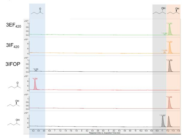
Analyzed using: Agilent Technologies 7890A GC system with column CP Chiralsil Dex CB (Agilent). Program: 40 °C to 140 °C in 5 min, 140 °C to 40 °C in 10 min.
