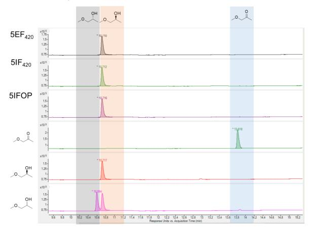
Analyzed using: Agilent Technologies 7890A GC system with column FS-Hydrodex-B-TBDAc (Aurora Borealis) Program: 40 °C to 190 °C in 5 min, 190 °C to 40 °C in 10 min.
