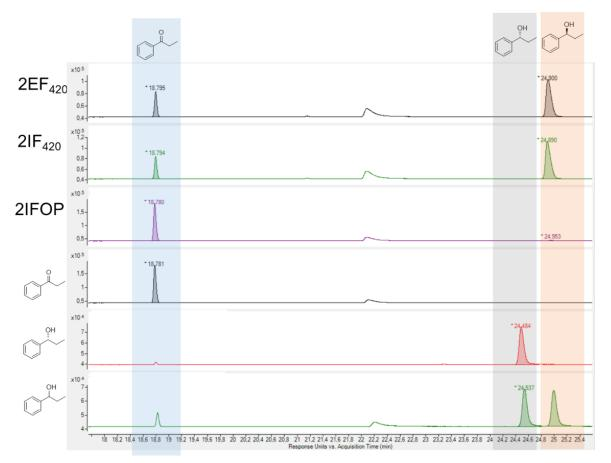
Analyzed using: Agilent Technologies 7890A GC system with column CP Chiralsil Dex CB (Agilent). Program: 40 °C to 120 °C in 3 min, 120 °C to 40 °C in 10 min.
