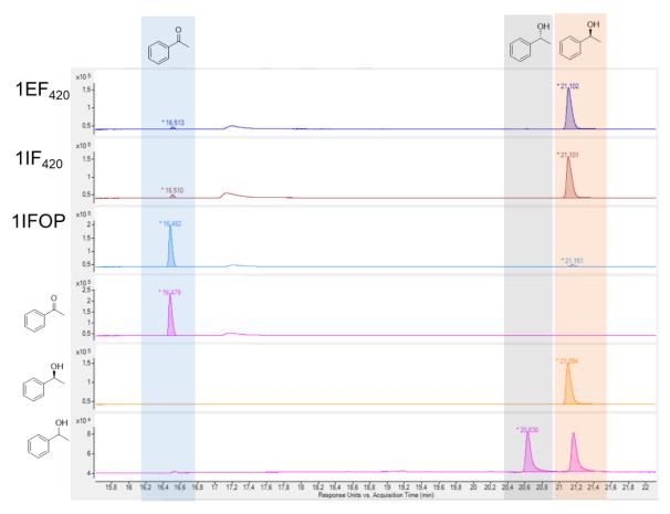
Analyzed using: Agilent Technologies 7890A GC system with column CP Chiralsil Dex CB (Agilent). Program: 40 °C to 130 °C in 5 min, hold 130 °C 10 min, 130 °C to 180 °C in 10 min, hold 180 °C in 5 min.
