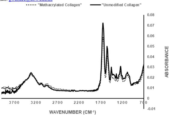
Figure 1. Comparison of FTIR spectra of extracted marine-derived collagen with (dotted line) and without (solid line) methacrylation. Samples were tested as freeze-dried foams at room temperature
