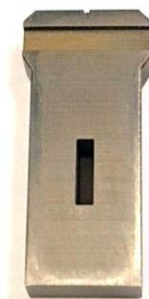
Figure S3 Example of apertures to be inserted into the collimator. a) standard aperture and b) an aperture with integrated photodiode for alignment.
