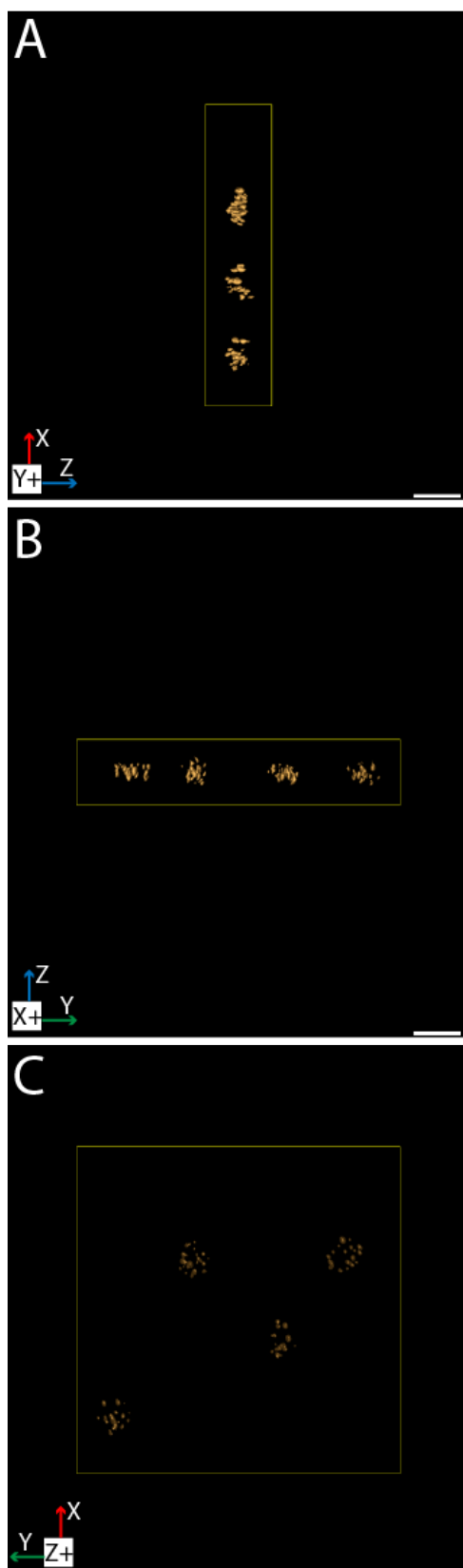
Figure S14: Tomography reconstruction of G7-Au based DENdroids.(A) XZ isosurface, (B) YZ isosurface, (C) XY isosurface. Scale bars represent 25 nm.
