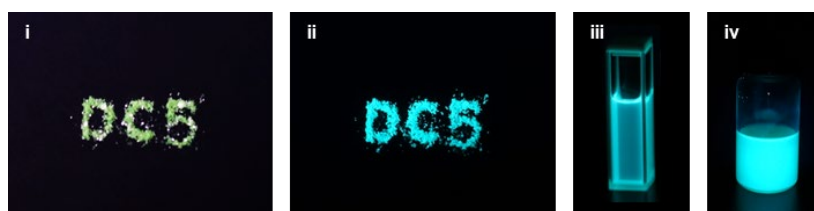
Supplementary Fig. 3 Photographs of DC5 crystal under white light (i), upon UV irradiation (ii), and in THF solution ( c = 10^{-4} M) upon UV irradiation (iii). A Photograph of fluorescent LC mixture (0.25 wt % DC5 in LC host E7) upon UV irradiation (iv).
