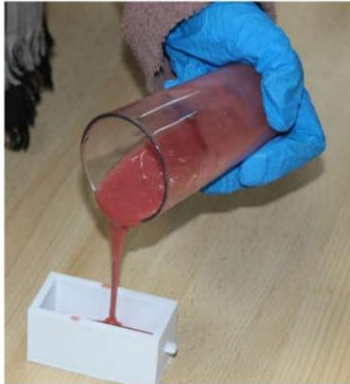
Fig. S5. Preparation of silicon rubber. (A) Mixture of base material and hardener before mixing. (B) Material after mixing. (C) pour the material in the mold.
