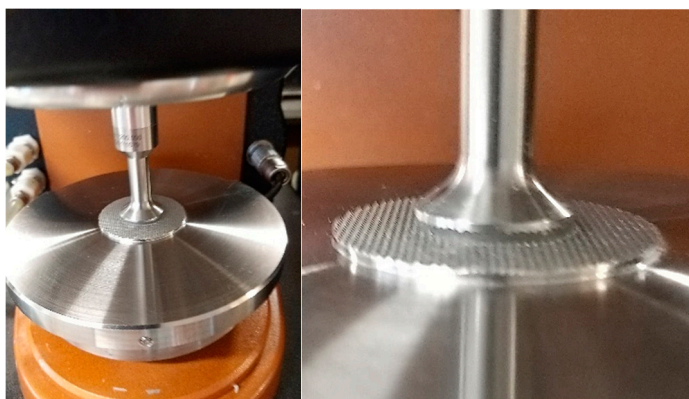
Figure S5. Sample loading in a rheometer, 1 mm gap size, removal of the extra sample outside the geometry and of the solvent trap.
