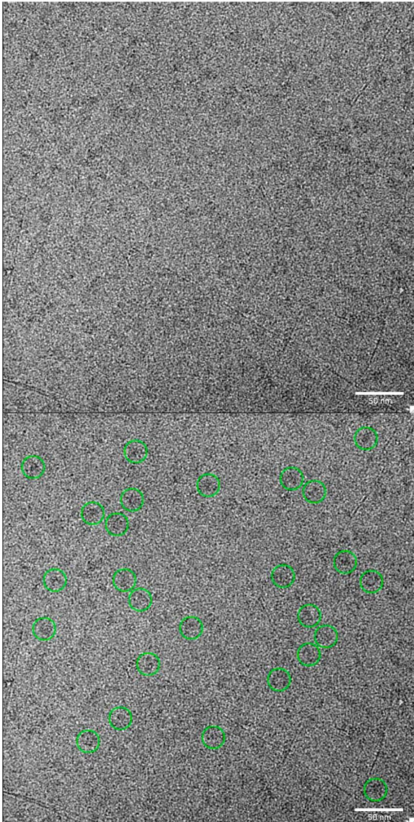
**Supplementary Fig. 19:** Representative micrographs of FADD:Caspase-8:FLAG-c-FLIP<sub>s</sub> complexes collected by Cryo-EM. In each case, top image shows unpicked micrograph, bottom image particles picked (green circles) from micrograph by CrYOLO. A single dataset was collected by CryoEM for this complex. These complexes are representative of those on
