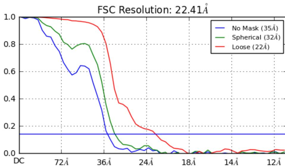
**Supplementary Fig. 5:** FSC Curve for Negative-stain dataset of FLAG-FADD:Caspase-8 complexes analysed using CryoSPARC v2.1.
