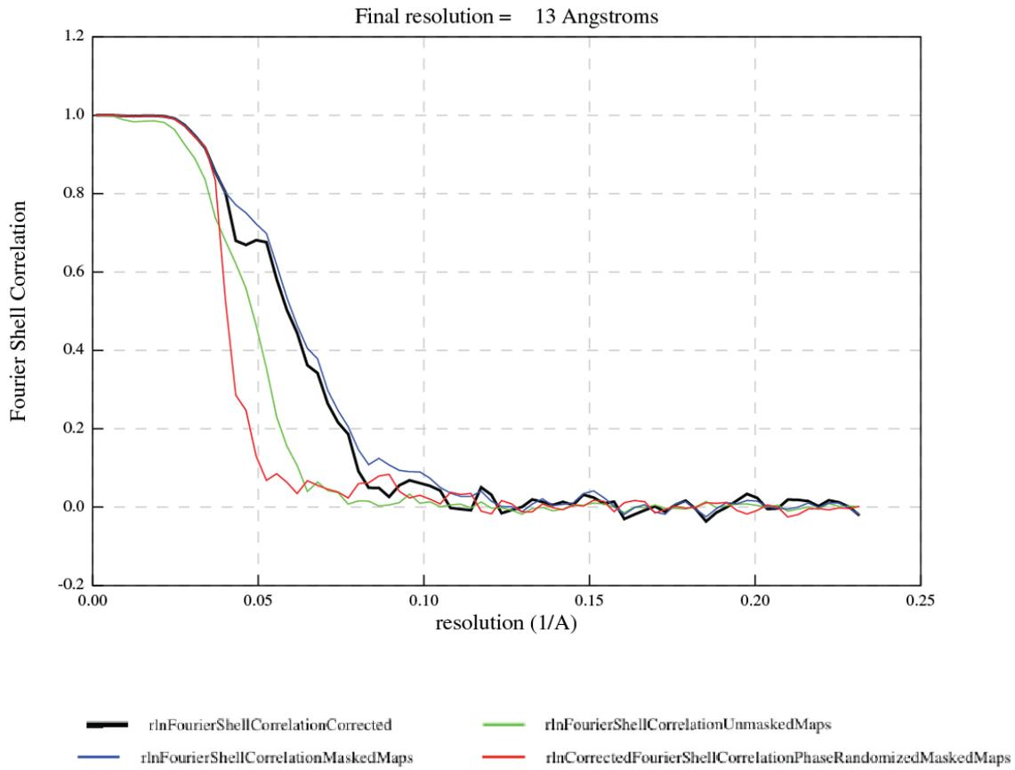
**Supplementary Fig. 18:** FSC Curve for single particle analysis of FADD:Caspase-8:FLAG-c-FLIP<sub>s</sub> complex dataset collected by Cryo-EM and processed in RELION 3.
