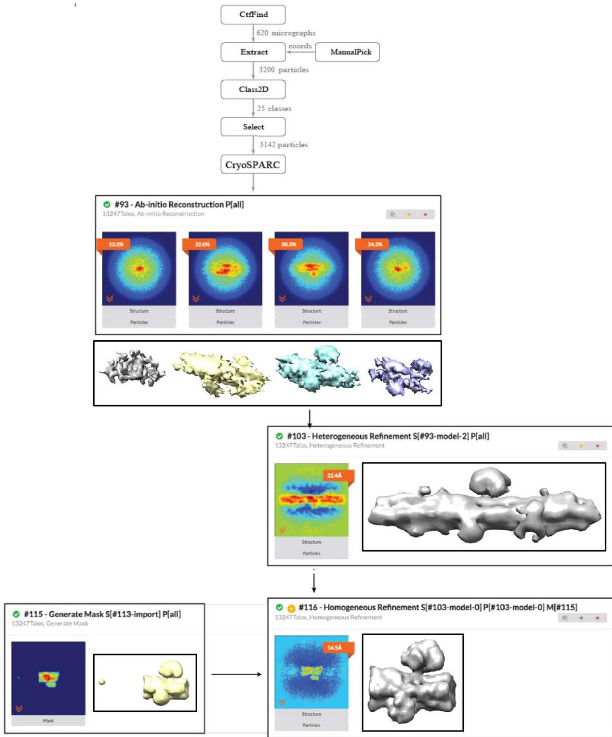
**Supplementary Fig. 4:** Flowchart of single particle analysis of Negative-stain dataset of FLAG-FADD:Caspase-8 complexes in RELION and CryoSPARC. 3D Volumes are shown in grey.
