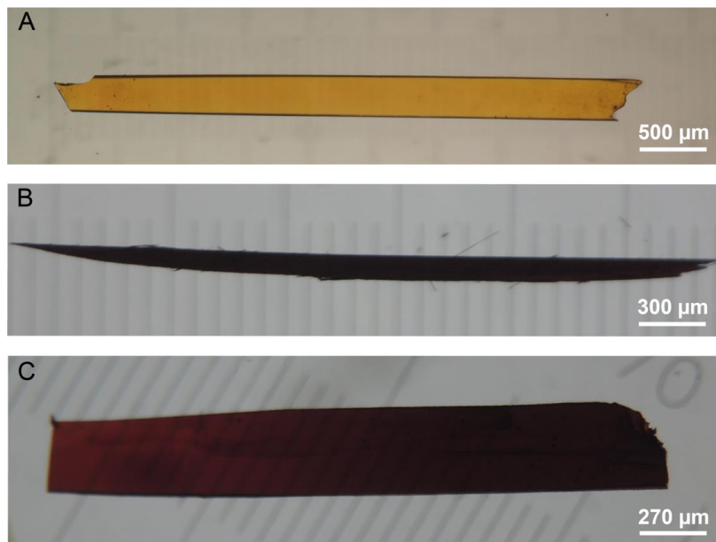
Fig. S1. Optical image of typical single crystals of (a) DDAB, (b) DMNAB, and (c) DR1.
