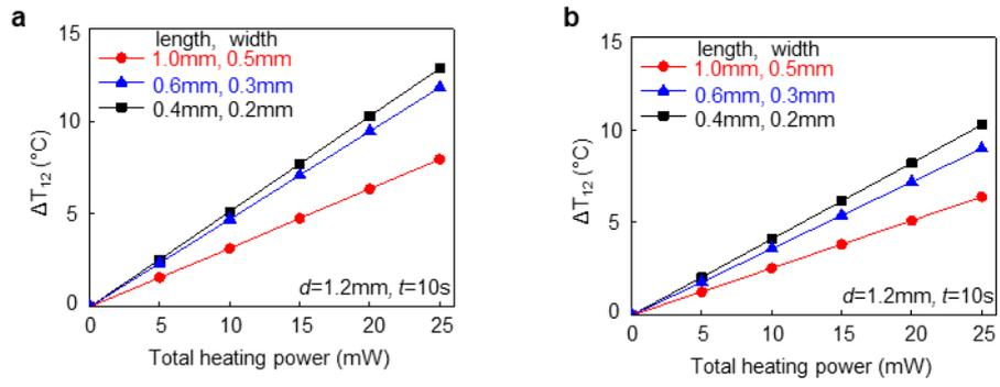
**Figure S6.** Computational prediction of  $\Delta T_{12}$  with different sizes of actuators (width and length of  $R_H$ ) for 30 % (a) and 95 % (b) hydrated skin.
