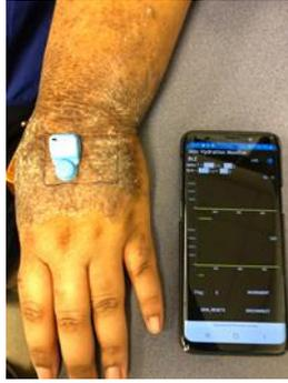
**Figure S20.** Optical image of the device mounted on the atopic hand of a subject 1, next to a BLE-enabled smartphone.
