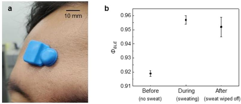
**Figure S19. a.** An optical image of the device mounted on the forehead of a healthy male subject. **b.** Wireless measurements of  $\Phi_{BLE}$  before, during and after a workout. Vertical bar denotes the error bar over 3-time measurements.
