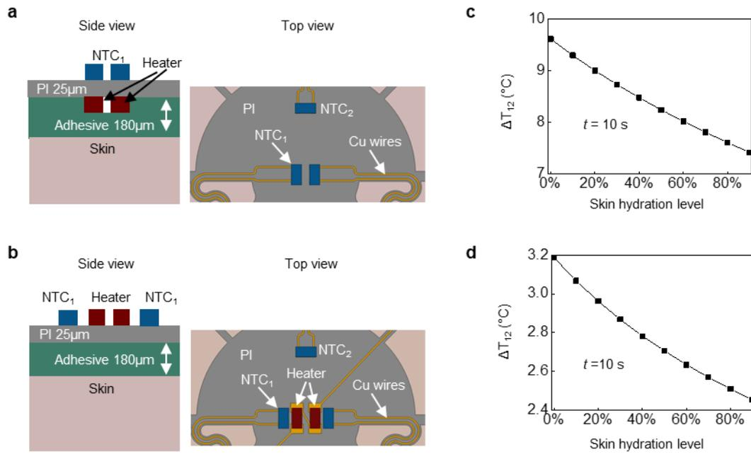
**Figure S3. a,b.** Schematic illustration of the FEA model of dual-sided (**a**) and single-sided (**b**) sensor designs. **c,d.** Sensitivities of the temperature difference ( $\Delta T_{12}$ ) between NTC<sub>1</sub> ( $\Delta T_1$ ) and NTC<sub>2</sub> ( $\Delta T_2$ ) to skin hydration level of dual-sided (**c**) and single-sided (**d**) designs 10 s after the heater is activated.
