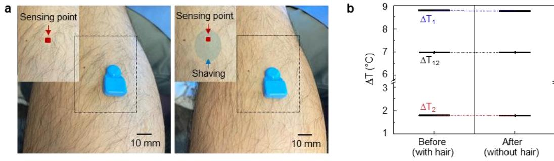
**Figure S18. a.** Pictures of the device on a subject's leg before (left) and after (right) shaving the skin. Insets show the sensing point. **b.** Wireless measurements of  $\Delta T_1$  (blue),  $\Delta T_2$  (red), and  $\Delta T_{12}$  (black) before and after shaving the sensing area.
