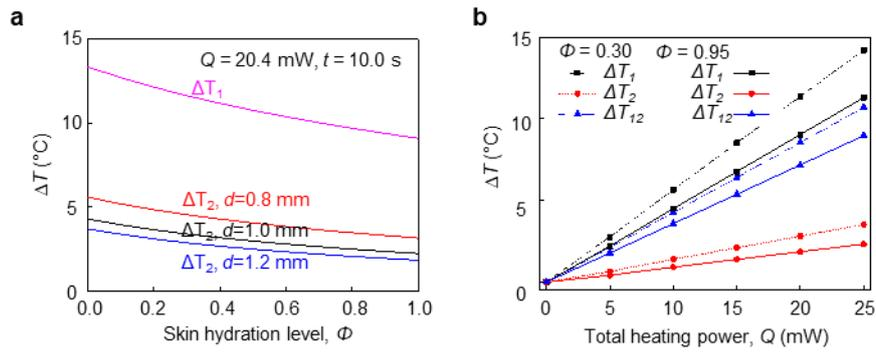
**Figure S5.** Computational predictions of  $\Delta T$  as a function of skin hydration level ( $\Phi$ ) with different values of  $d$  (**a**;  $Q = 20.4 \text{ mW}$ ,  $t = 10.0 \text{ s}$ ), and  $\Delta T$  as a function of  $Q$  (**b**;  $d = 1.2 \text{ mm}$ ,  $t = 10.0 \text{ s}$ ).
