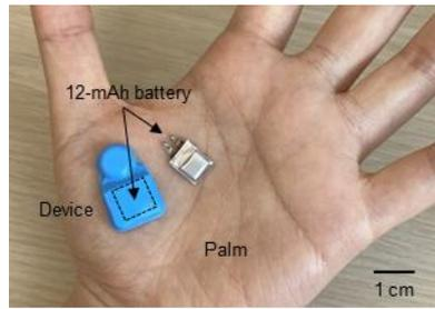
**Figure S1.** Picture of an encapsulated device next to a 12 mAh Li-polymer battery.
