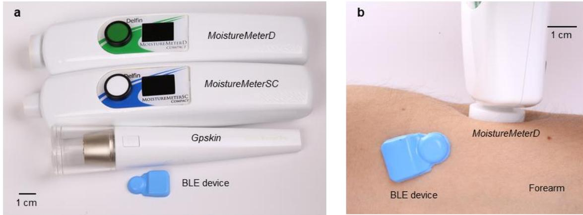
**Figure S9. a.** Picture of conventional devices based on skin capacitance measurements for monitoring tissue water content (*MoistureMeterD*; top), SC hydration levels (*MoistureMeterSC*; middle top), and skin surface hydration levels (*Gpskin*; middle bottom), and a BLE device (bottom). **b.** Picture of devices on the forearm. The commercial devices require care by the user to hold the probe and apply a certain pressure against the skin for each measurement.
