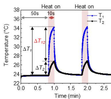
**Figure S2.** Wireless read-out of the temperature change measured from NTC<sub>1</sub> ( $\Delta T_1$ ) and NTC<sub>2</sub> ( $\Delta T_2$ ) as a function of time for 10 s of heating every one min.  $\Delta T_{12} = \Delta T_1 - \Delta T_2$ .
