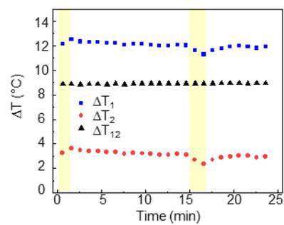
**Figure S8. Ambient temperatures.** Measurements of  $\Delta T_1$  (blue),  $\Delta T_2$  (red), and  $\Delta T_{12}$  (black) as a function of time (min). The values of  $\Delta T_1$  and  $\Delta T_2$  fluctuate at the moment the device enters and exits the oven (yellow background).
