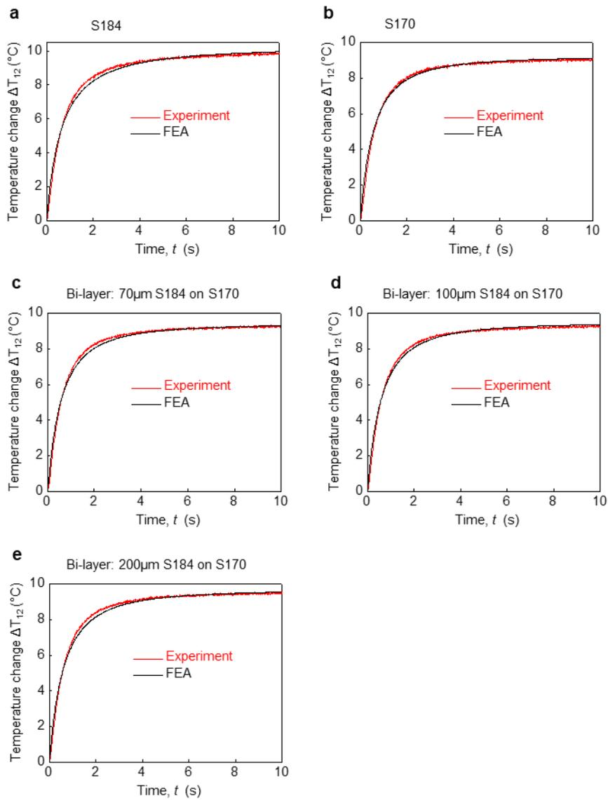
**Figure S4.** Comparison between FEA and measurement for a thick layer of S184 (a) and S170 (b), and a thin layer of S184 (70  $\mu$ m, c; 100  $\mu$ m, d; 200  $\mu$ m, e) on top of the S170.
