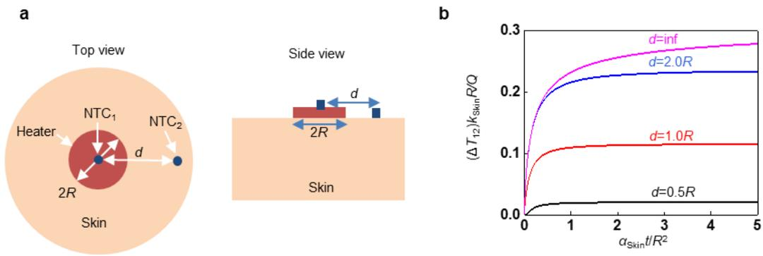
**Figure S7. Effect of design parameters on the temperature change. a.** A simplified, analytical model of a disk-shaped thermal actuator (radius,  $R$ ) and NTCs. **b.** Analytical scaling law for  $\Delta T_{12}$
