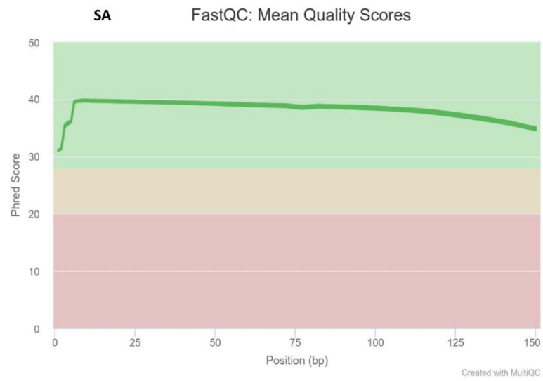
Supplementary Figure 2: Mean sequencing Phred scores of > 35 was achieved in the WES data.
