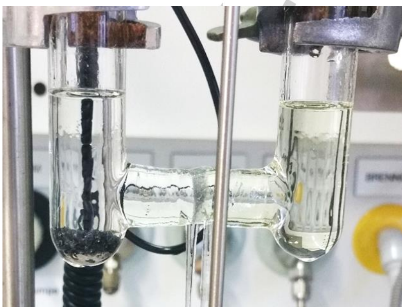
Figure S6. Picture of the diffusion experiment with needles of Ag_2Te grown on the the silver (left side) and Te (right side) in [P_{6614}]Cl after one week at 200 °C.
