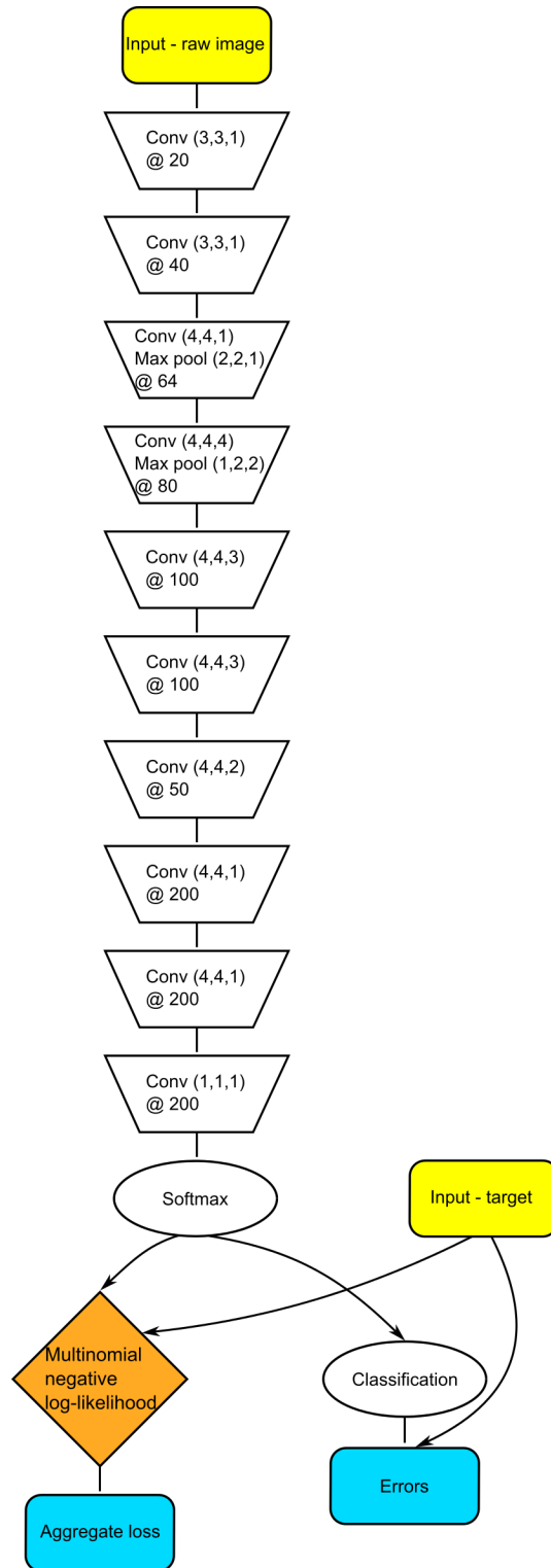
Supplementary Figure S7. The architecture of DCNNs used in DeepACSON. We used the same architecture for DCNN-m Ax and DCNN-cN. The size of the convolutional kernels is denoted as Conv(x,y,z) . The number of channels/feature maps created from a layer of convolutional kernels is denoted by @ n . The size of the max pooling operation is denoted as Max\ pool(x,y,z) .
