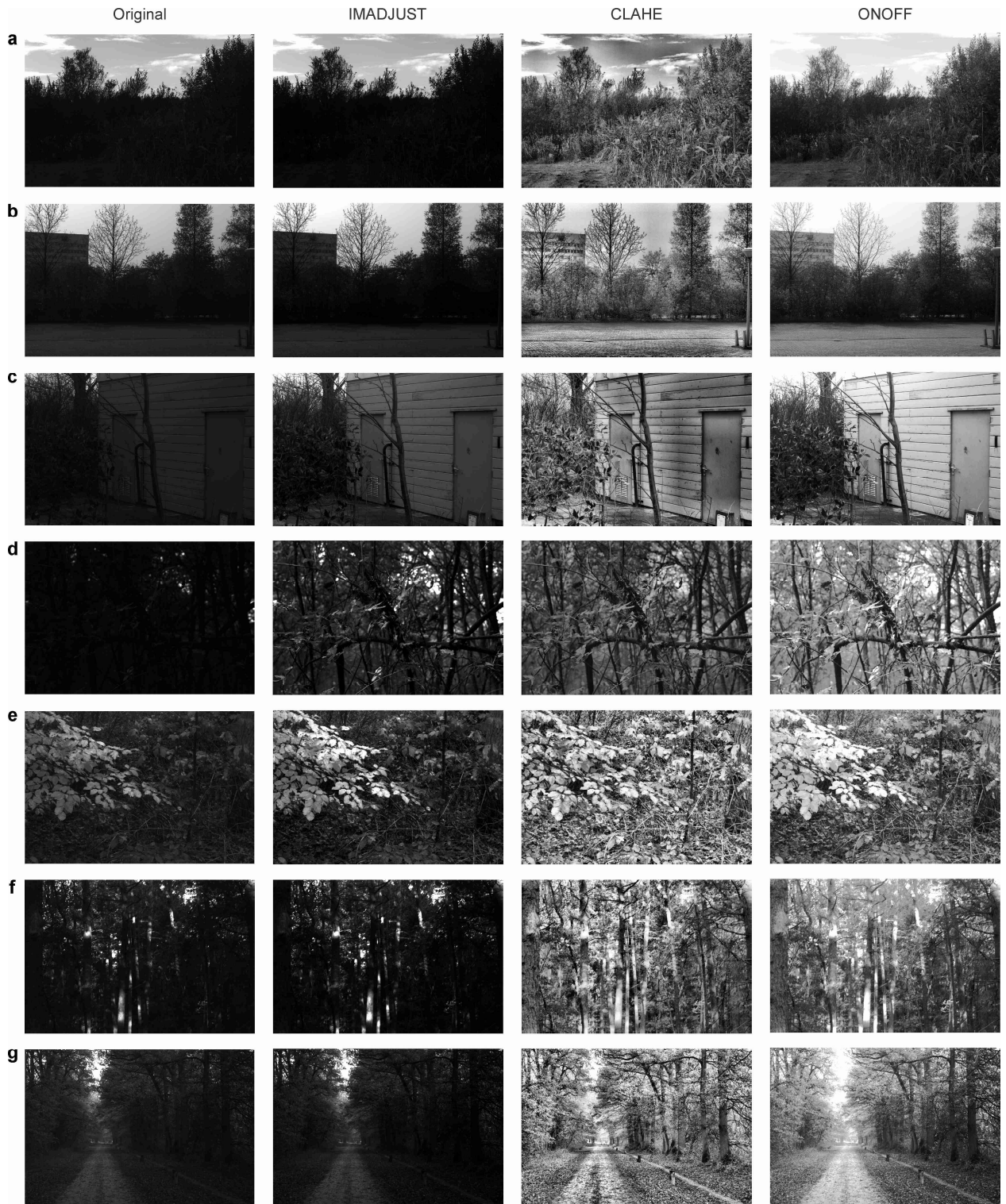
Supplemental Figure 4. Images processed with three different algorithms to simulate human luminance vision. a. From left to right, original image, image processed with Matlab image adjustment (IMADJUST), contrast-limited adaptive histogram-equalization (CLAHE), and the ONOFF algorithm. b-g. Same for other example images. The images processed with the ONOFF algorithm reproduce more closely human perception, particularly when the images have bright sky patches. Original images from (van Hateren and van der Schaaf, 1998). Related to Figure 7.
