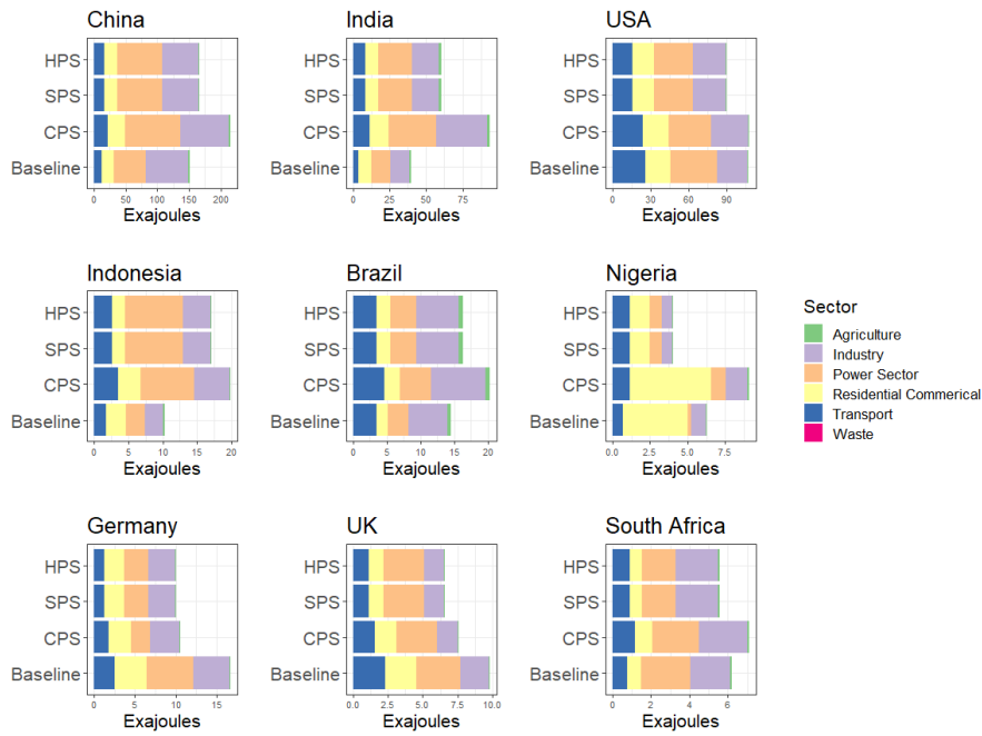
Figure S4. Total primary energy supply (TPES) by sector for each country in 2015 and under future (2040) scenarios
