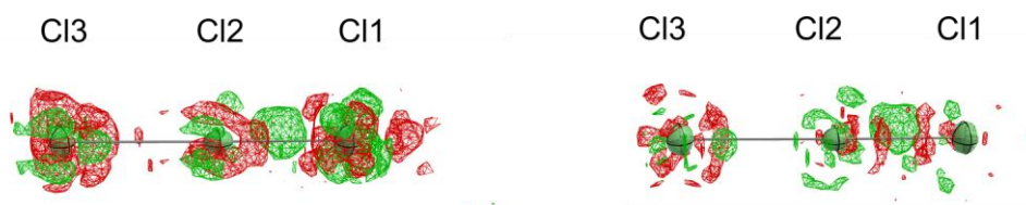
Figure S12. Residual density before and after anharmonic refinement. The isosurface value is \pm 0.06 \text{ e}\text{\AA}^{-3} . Positive contours are plotted with green lines and negative contours are plotted with red lines. The graphics were created with MoleCoolQT [19] .
