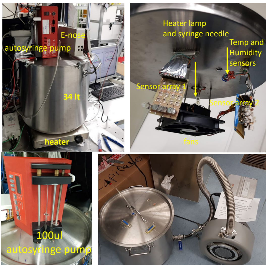
Figure S2: Photographs of the experimental setup. The individual components are labelled. The experiments were performed with sensor array 2 (picture top right). The circuit board of this sensor array has a size of 6 cm × 9 cm and the QCM sensors point up to 2 cm out, so the total volume of the sensor array is about 100 cm 3 .
