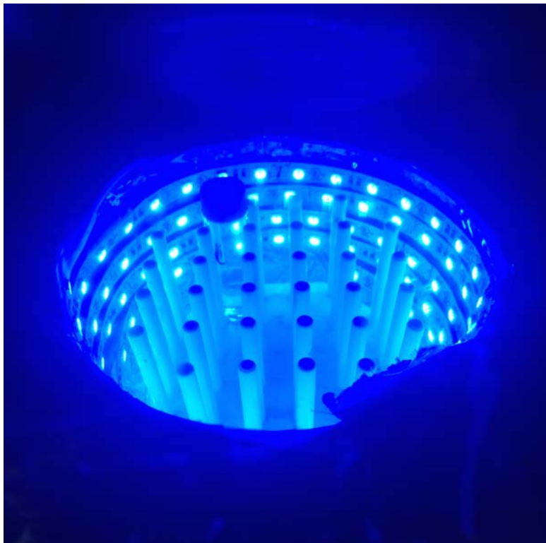
Figure S23. Reaction set-up using blue LEDs.
