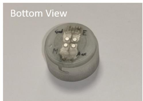
Figure 5. EMG /ECG BT device overview and pictures at different stage of assembly.
