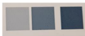
Figure 3. Example of samples obtained by printing PEDOT:PSS Clevis P Jet 700 as received on washed Silhouette tattoo paper (top), and samples obtained by printing PEDOT:PSS Clevis P Jet with addition of 10% vol of glycerol (bottom). Typical value for electrodes' surface resistivity are reported.
