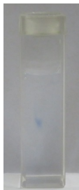
Supplementary Fig. 41 Photograph of \text{Eu}^{3+} -L-CF-1 aqueous solution that was firstly irradiated with visible light ( >450 nm) for 15 s, and then measured by luminescence analyzer ( \lambda_{\text{ex}} = 265 nm).
