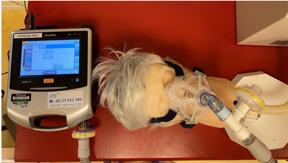
e-Figure 1: 3D-printed head model with setup 4 test.
