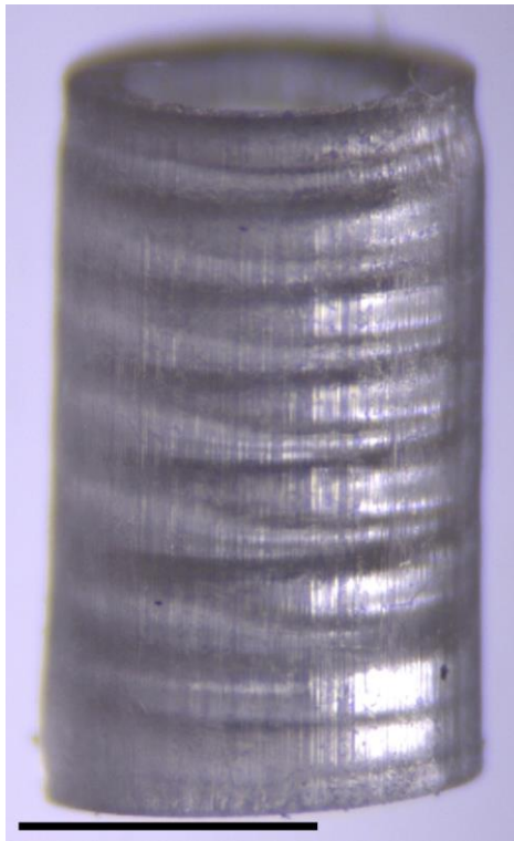
Figure S1. Optical microscopy image of a PCLMA tube produced via microstereolithography with non-optimal curing conditions. Lateral ridges can be seen due to overcuring of the material as a result of high laser power and the higher viscosity of room temperature resin. Scale bar: 1 mm.
