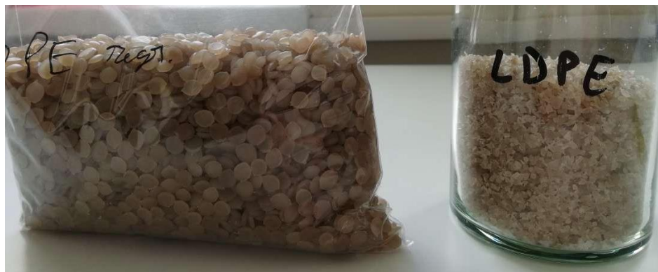
Figure S1. Pellets (left) of recycled LDPE (recyclate of transparent mostly label-free packaging film) and the fragments (right) from the first milling (Retsch SM100). For the current study, fragments from the first milling were further milled into smaller (<500 \mu\text{m} ) fractions (Figure S2).
