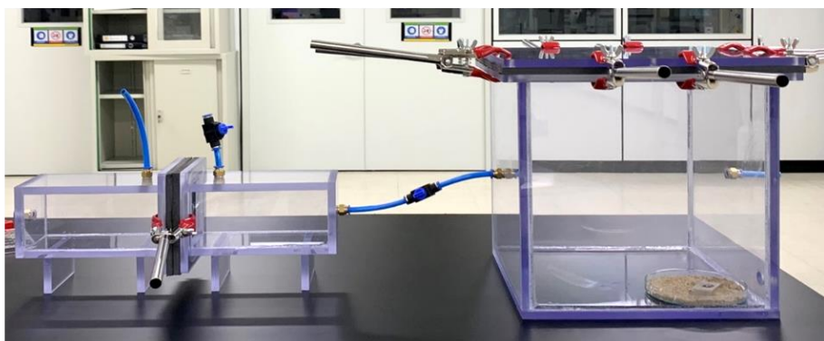
Figure S2. Setup used to measure pressure drop and removal efficiency.
