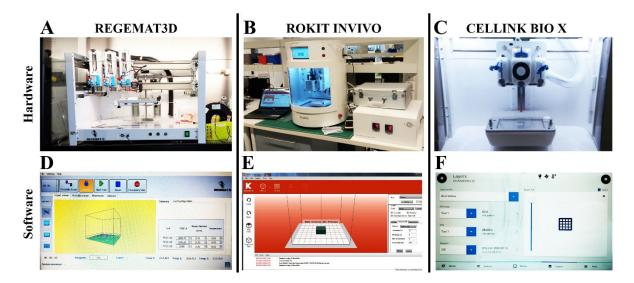
Supplementary Figure 1. 3D bioprinting platforms used: a custom-made REGEMAT3D model (left column), the ROKIT INVIVO (middle column) and the CELLINK BIO X (right column). Hardware (A-C) and software (D-F) are shown for these three extrusion-based 3D bioprinting systems. The REGEMAT3D customised (D) and INVIVO 'Creator K' (E) software were both accessed on a laptop computer connected to the bioprinter by USB cable and the BIO X software (F) was entirely inbuilt on the bioprinter touchscreen.
