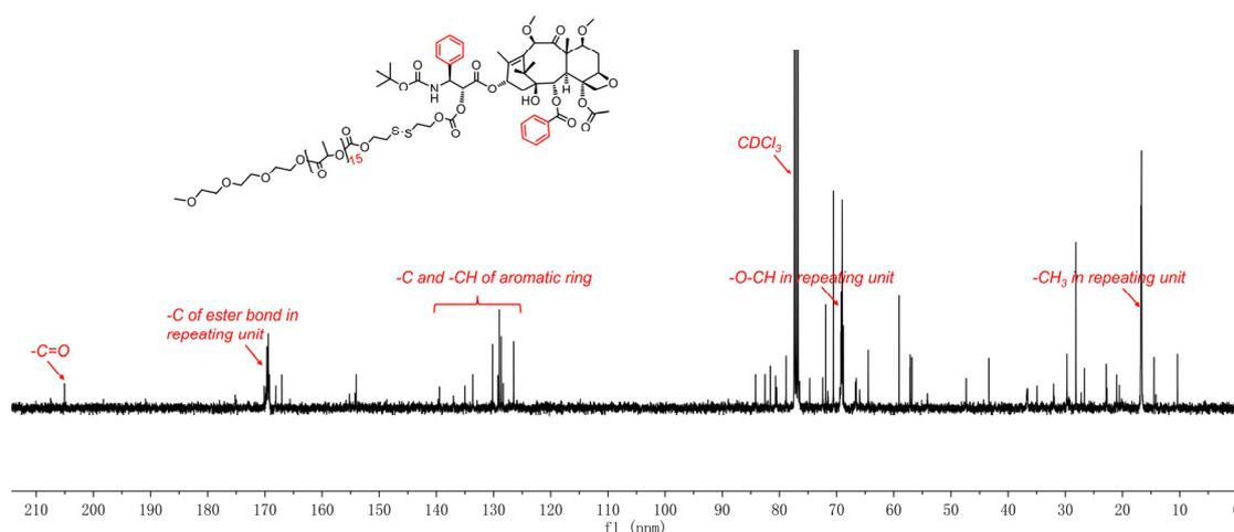
**Figure S7.**  $^{13}\text{C}$  NMR spectrum of pLA<sub>15</sub>-SS-CTX conjugate in  $\text{CDCl}_3$ .
