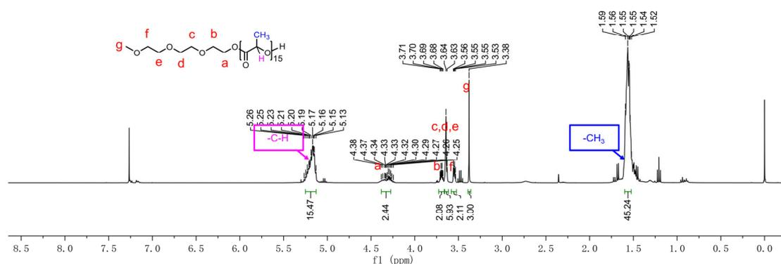
**Figure S1.**  $^1\text{H}$  NMR spectrum of hydroxyl-terminated polylactide ( $\text{pLA}_{15}$ ) in  $\text{CDCl}_3$ .
