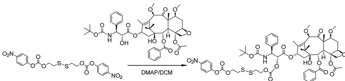
The conjugate **1** (0.50 mmol, 244.14 mg) and 4-dimethylaminopyridine (DMAP, 0.57 mmol, 70.15 mg) were dissolved in 4 mL of DCM. Under stirring at  $45^\circ\text{C}$ , a solution of cabazitaxel (0.48 mmol, 400 mg) in 2 mL of DCM was added dropwise into the mixture. After stirring for 30 min, the
