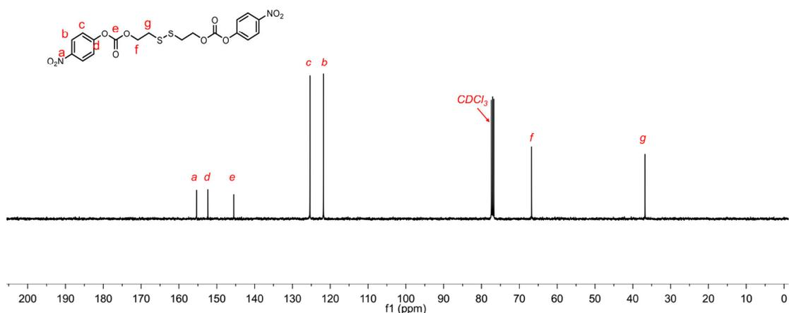
**Figure S4.**  $^{13}\text{C}$  NMR spectrum of the conjugate **1** in  $\text{CDCl}_3$ .
