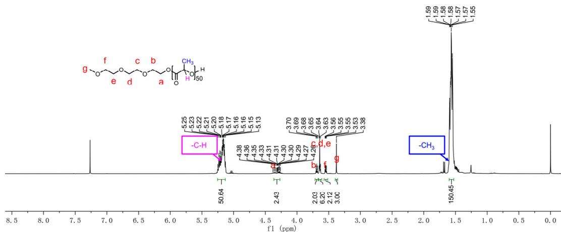
**Figure S2.**  $^1\text{H}$  NMR spectrum of hydroxyl-terminated polylactide ( $\text{pLA}_{50}$ ) in  $\text{CDCl}_3$ .
