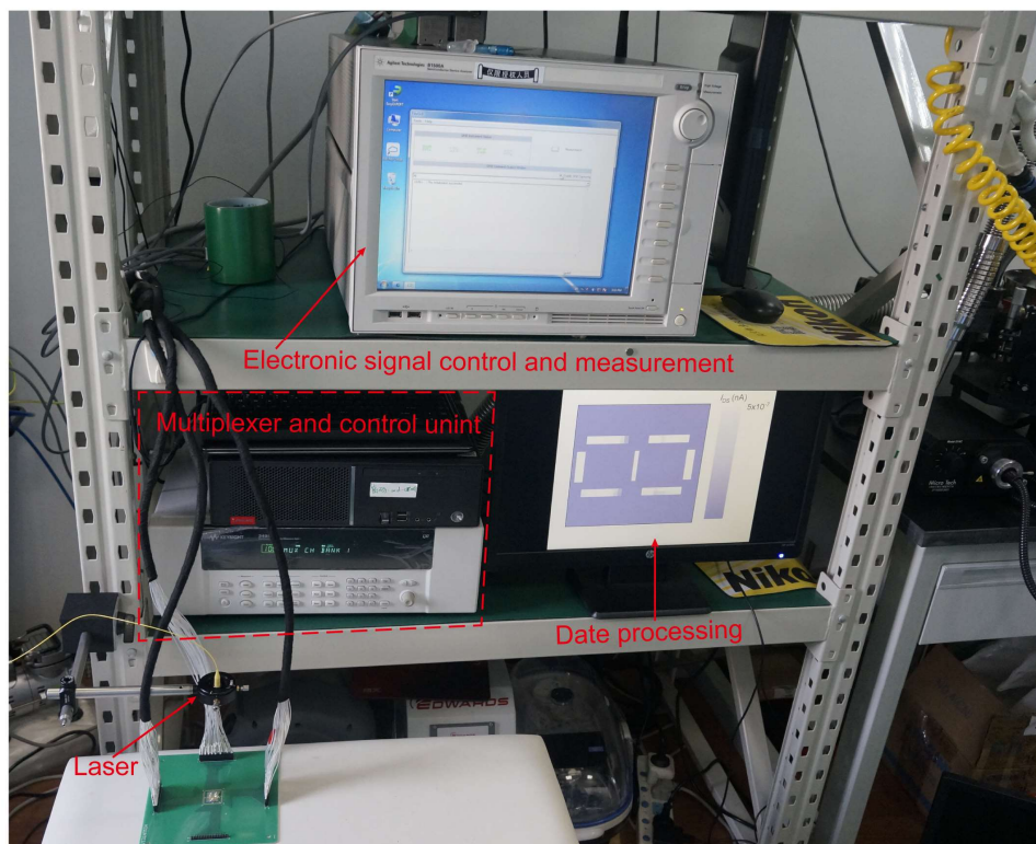
Supplementary Fig. 33 Photograph of the measurement system for the optoelectronic sensor array . The system contains four parts: (i) laser, (ii) multiplexer and control unit, (iii) electrical signal control and measurement, and (iv) data processing.
