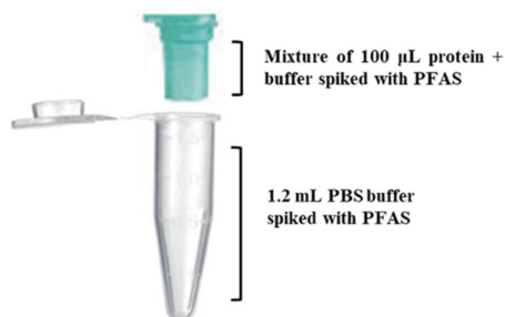
Figure S1. Equilibrium dialysis setup with materials used (dialysis filters and vials) shown.
