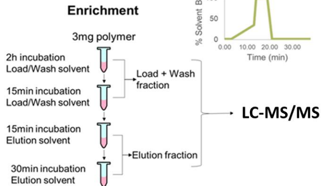
Figure S12: Schematic representation of the workflows. a) Three short phosphopeptides were first spiked in BSA+ B-Casein digest in two spiking levels (1:10 and 1:20) before SPE. Load+Wash and Elution fractions were collected and dried prior LC-MS/MS analysis. b) Protein digests were first de-salted and dried prior MIP SPE. Load+Wash and Elution fractions were collected and dried prior LC-MS/MS analysis.
