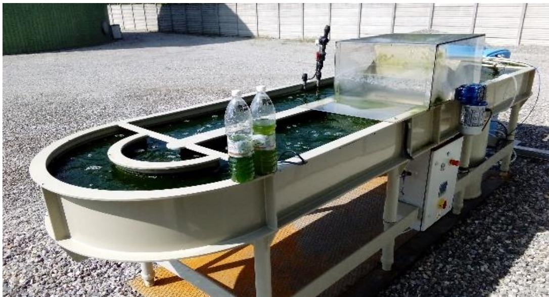
22 Figure SI.1.1. Scheme of the pilot-scale HRABP setup (A); picture of the pilot-scale HRABP (B).
