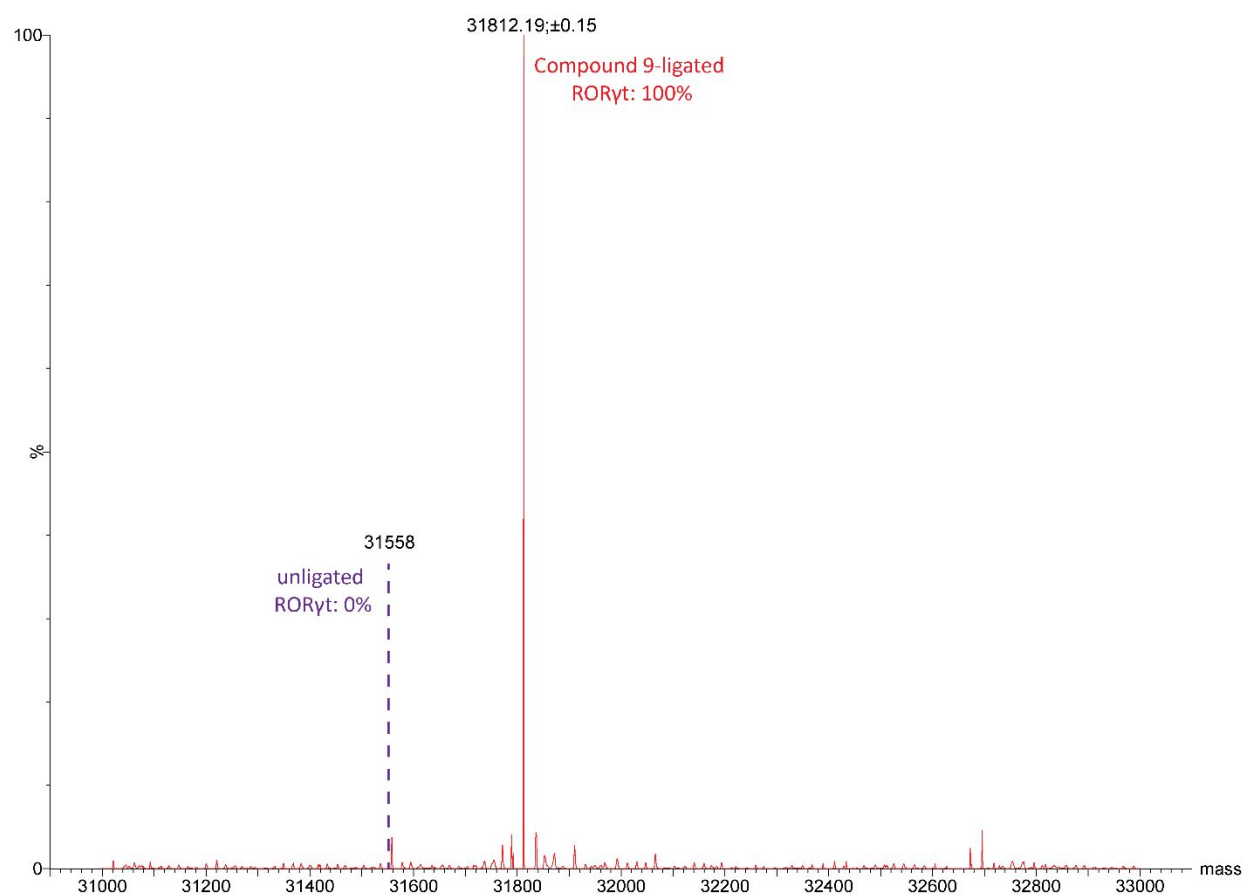
Figure S7. Deconvoluted Q-TOF spectrum of ROR \gamma t ligated to compound 9 : 100% ligation is observed, while 0% unligated protein is visible (mass: 31558.11 Da). Mass expected: 31811.70 Da, mass observed: 31812.19 Da.
