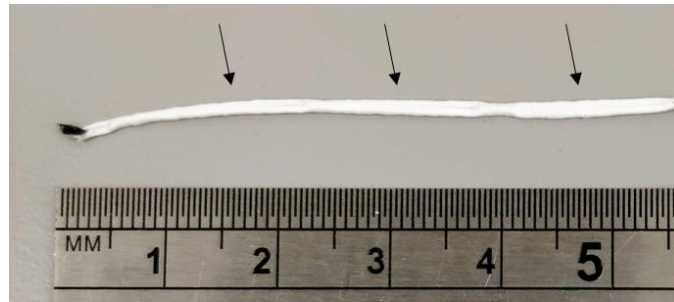
Figure S10. Photograph of triboelectric yarn after 200,000 tapping cycles. The arrows indicate the areas where tapping occurred. Note the increase in yarn diameter due to the deformation of the PVDF fibers.
