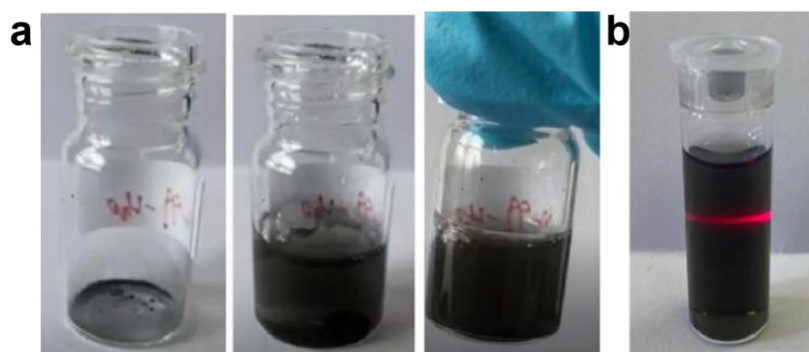
Figure S3. (a) the delamination of I_2 -etched Ti_3AlC_2 in 1.0 M HCl by manual shaking and (b) the aqueous dispersion of 2D IE-MXene.
