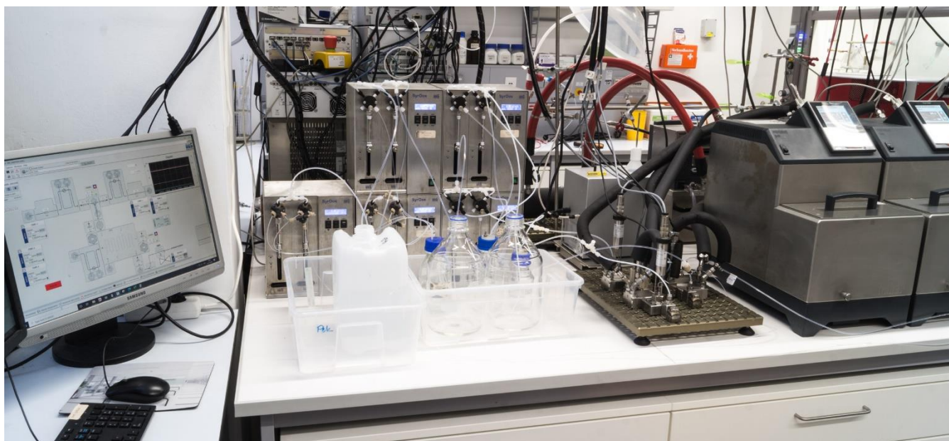
Figure S43. Photograph of the nitration setup.
