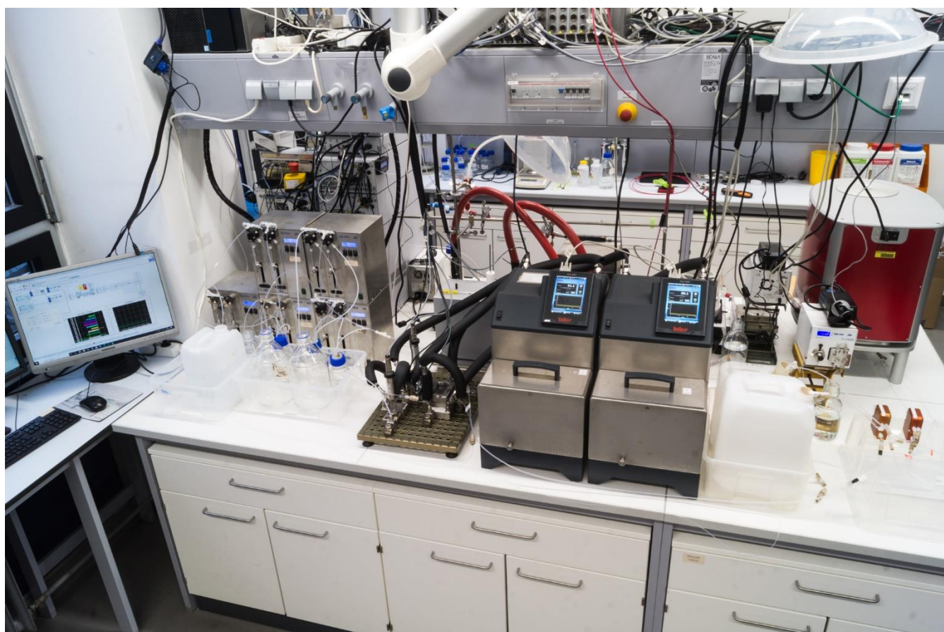
Figure S2. Photograph of the nitration and extraction setup.
