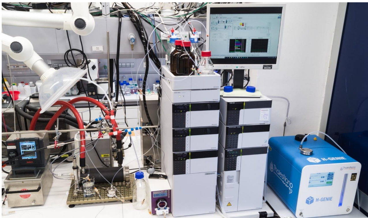
Figure S81. Photograph of hydrogenation setup.
