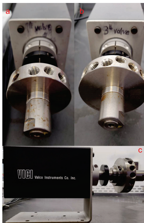
Supplementary Figure 4. Photograph of the multiway selector valves. a, 10-position selector valve, VICI EUTA-2SD10MWE. b, 16-position selector valve, VICI EUTA-2SD16MWE. c, Profile view of the selector valve.
